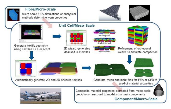
The software can be used both via a user interface and a Python scripting API. Developed within the Composites Research Group at the UoN it is typically used as shown above but has been designed to be flexible so that a wide range of textile forms can be modelled.
